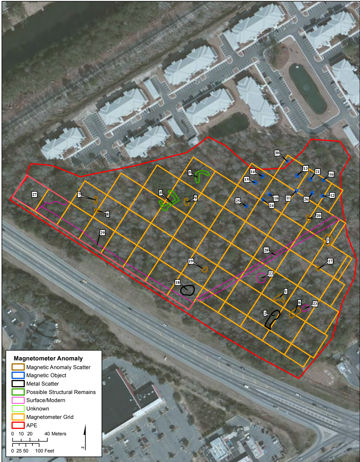
Figure 27. Magnetic Anomalies Within the Project Area
